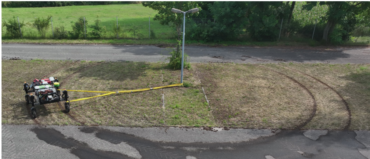
Figure 3: Curve test setup. The Tipard 350 is attached to a fixed point via lifting slings and is thus held on a fixed circular path (© Competence Centre for Digital Agriculture (KoDA) at the Weihenstephan-Triesdorf University of Applied Sciences)
