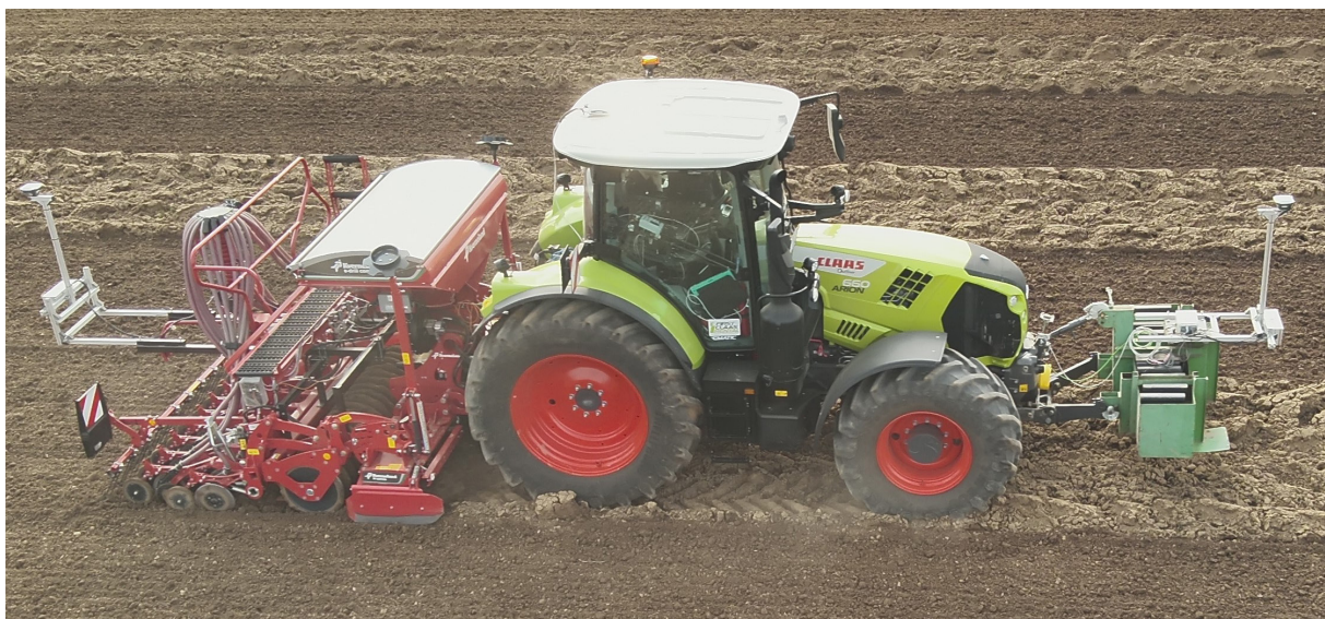
Figure 2: Kverneland e-drill compact attached to a Claas Arion 660 with a computer mounted in the cabin of the tractor and stereo cameras as well as GNSS antennas in the front and in the back of the machine (© Stein and Boysen)
