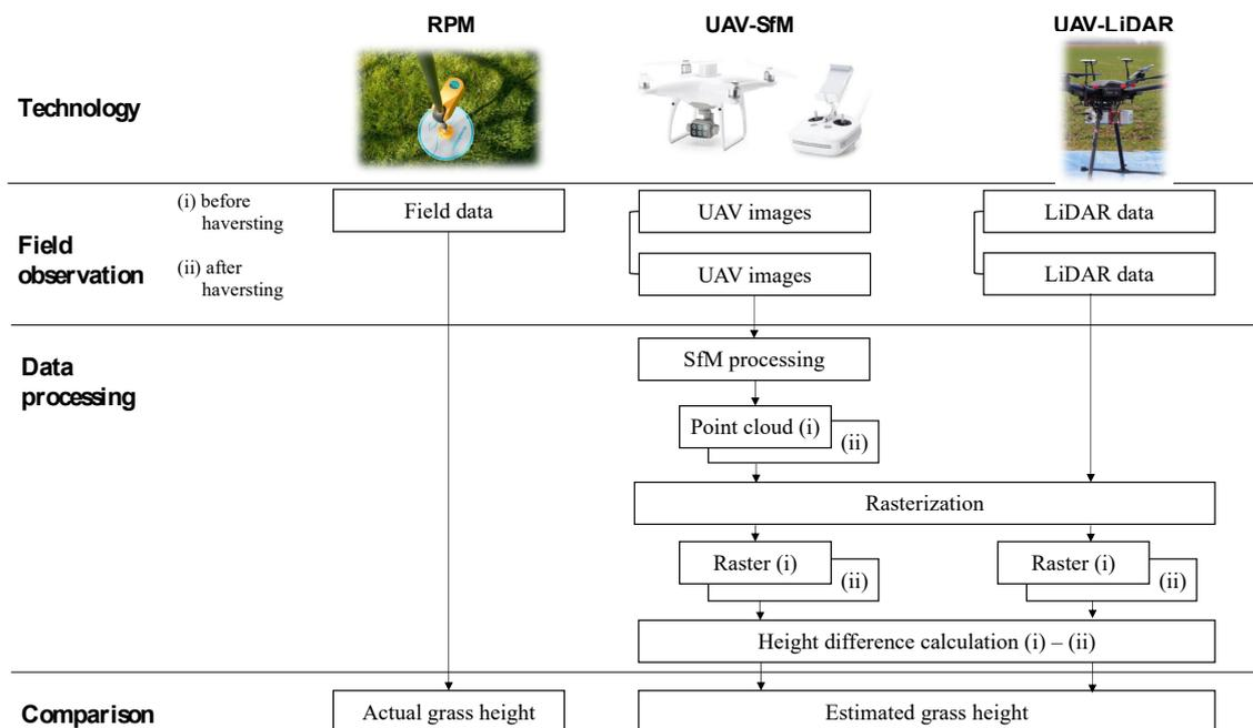
Figure 1: Outline of the measurement procedure (based on Obanawa et al. 2020)
