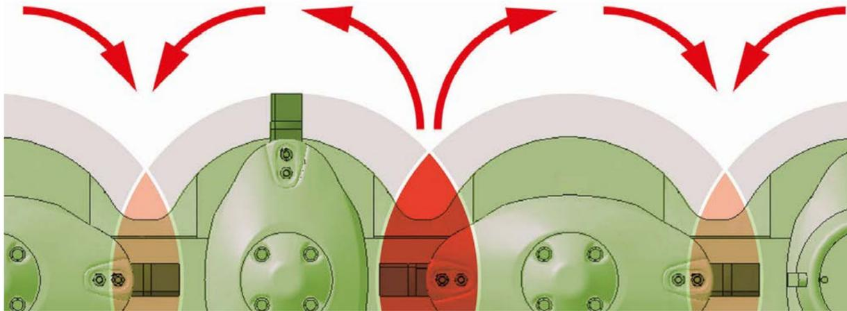
Figure 1: Top view of the overlapping zones of the KRONE EasyCut cutterbar; red arrows show the direction of rotation of the discs, orange zone = overlapping area where the blades move backward and red area = overlapping area where the blades move forward (MASCHINENFABRIK BERNHARD KRONE GMBH & Co. KG 2022)
