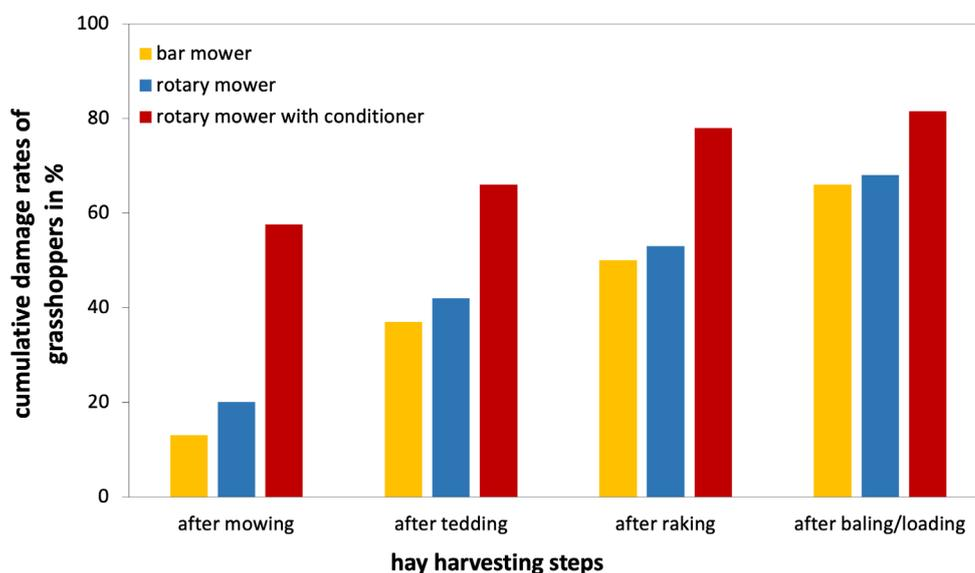
Figure 4: Cumulative percentage damage rates of grasshoppers in grassland after various harvesting steps with various types of mowing equipment. The values for the entire harvesting process were calculated from individual survival rates of the respective steps (HUMBERT et al. 2010a) and subsequently converted into damage rates.
