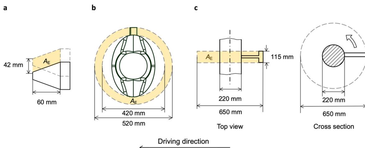
Figure 2: Top view of a) a double-blade mower and b) a disc mower, plus the top view and cross-section of c) a flail mower with the area  $A_E$  marked in yellow, which is influenced by the blade during a stroke or a revolution
