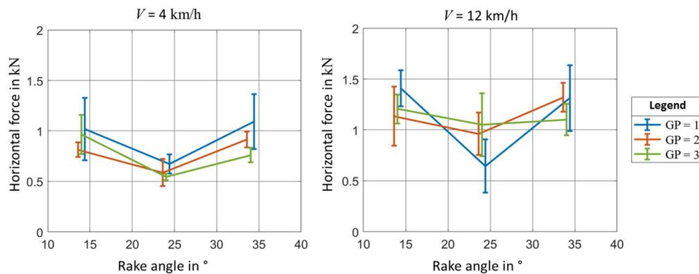
Figure 6.1: Draft force curves of the field tests; separated by speed for  $WD = 10$  cm
