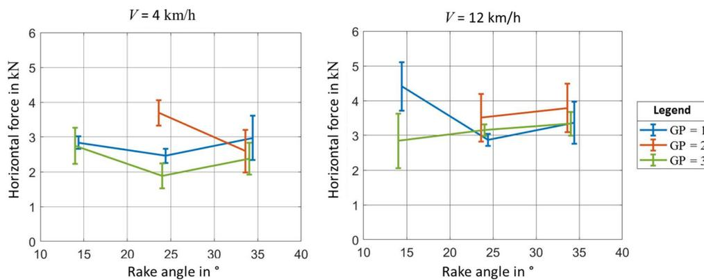
Figure 6.2: Draft force curves of the field tests; separated by speed for  $WD = 20$  cm
