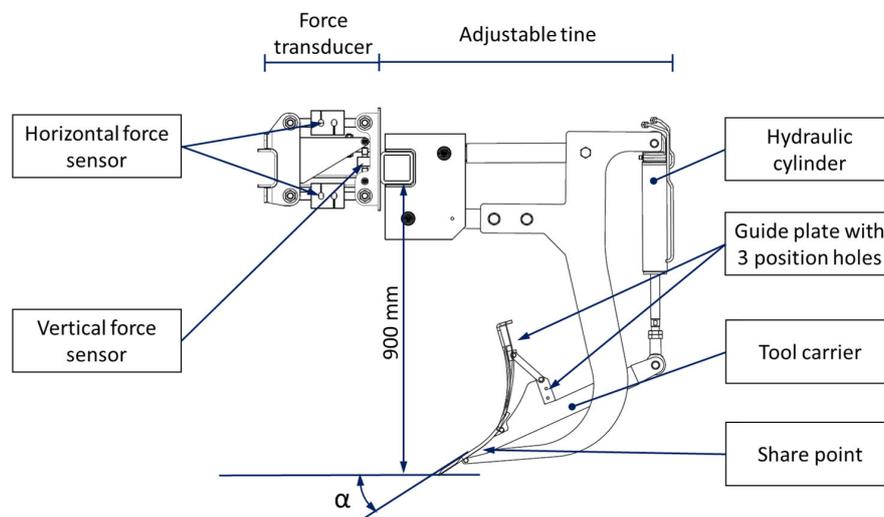
Figure 1: Cultivator tine with variable geometry and force transducer; rake angle  $\alpha = 34^\circ$ ; guide plate in position 1
