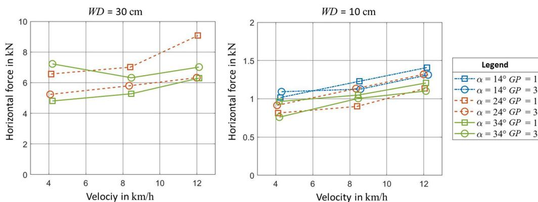
Figure 5: Curve array of horizontal forces of field tests for  $WD = 30$  cm and  $WD = 10$  cm
