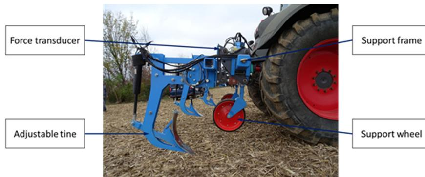
Figure 2: Field test set up with three adjustable tines
