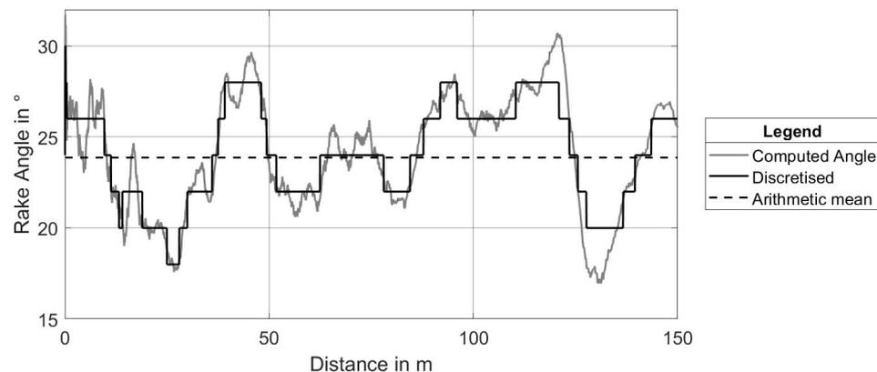
Figure 7: Graph of computed rake angle with minimal draft force
