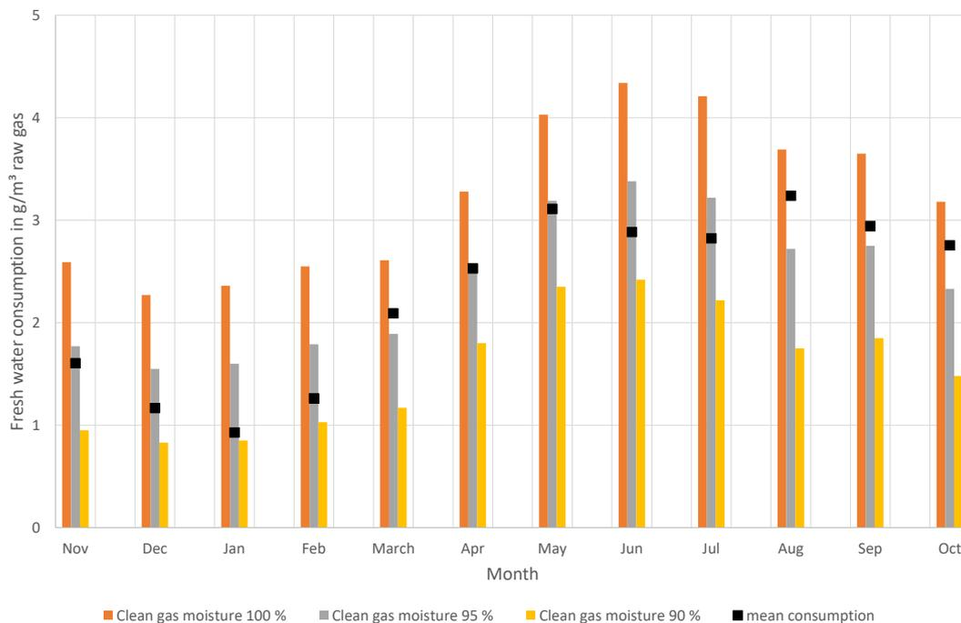
Figure 4: Monthly mean fresh water consumption of biofilters (n = 13) in comparison to calculated consumption rates for achieving humidity values of 90, 95 and 100% in the outlet
