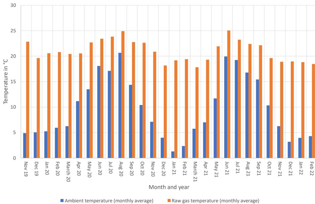
Figure 3: Course of monthly mean temperatures in ambient air and in the biofilter raw gas (n = 13)
