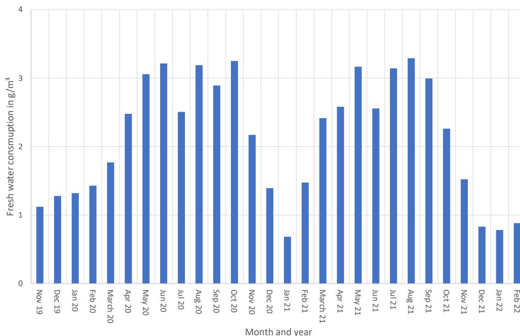
Figure 2: Mean fresh water consumption of biofilters per  $\text{m}^3$  raw gas during the year ( $n = 13$ )
