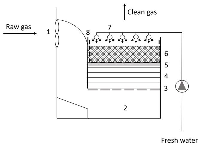
Figure 1: Schematic illustration of a single-stage biofilter for cleaning of exhaust air from pig stables without bedding with essential functional elements (fan (1); pressure chamber (2); supporting floor (3); wooden slats (4); recyclimate layer (5); biofilter material (6); humidification system (7) and freeboard (8))
