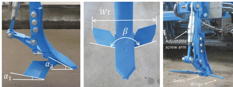
Figure 1: Adjustable tine wings: where:  $w_t$  wing width,  $\beta$  wing angle,  $\alpha_1$  wing rake angle, and  $\alpha_2$  tine rake angle
