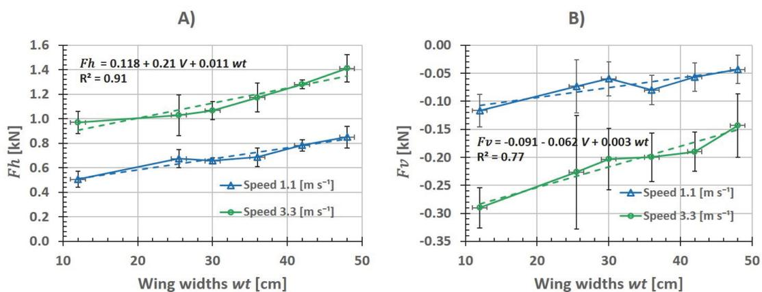
Figure 2: Effect of speed  $V$  and wing widths  $w_t$  on A)  $Fh$  and B)  $Fv$  ----- trend line (mean  $\pm$  SD)
