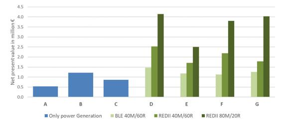
Figure 8: Comparison of the overall profitability of the seven connection scenarios for a 500  $kW_{el,inst}$  BGA – scenarios A to C with electricity generation only, D to F with proportional electricity and fuel production and G with complete fuel production
