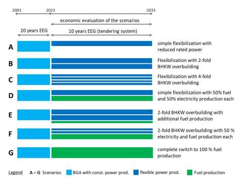
Figure 4: Seven connection scenarios for existing BGA after the end of the first EEG support period
