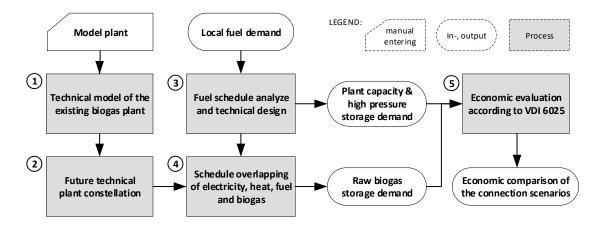
Figure 3: Five model components in the block diagram (represented as rectangular processes) for economic evaluation and comparison of the connection scenarios
