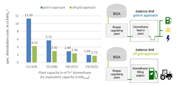
Figure 2: Specific cost comparison of the distribution approaches grid feed-in and off-grid approach for biomethane (grid feed-in costs from eMikroBGAA (BEIL and DANIEL-GROMKE 2019), off-grid costs own calculation)
