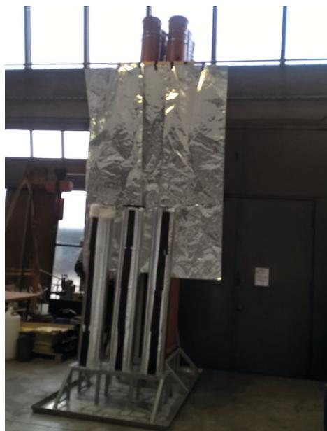
Figure 1: Experimental set-up for investigating the influence of stack height and particle size on the seepage formation of silage from chopped sugar beet (© Universität Hohenheim/S. Zielonka)
