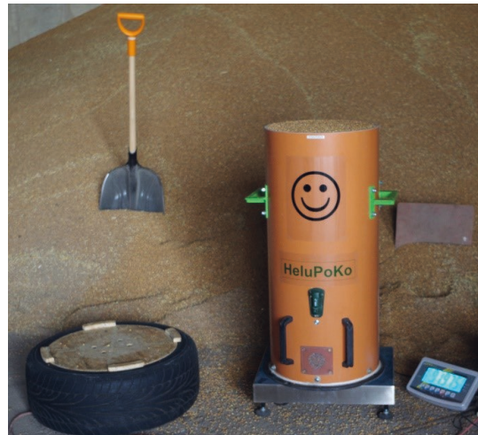
Figure 1: 100 litres vessel with vibration platform and scale to determine the weight of 100 litres grain (© J. Berberich)
