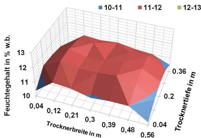
Figure 4: Average moisture content over the dryer cross section at outlet, measured in semi-technical scale, see Figure 1
