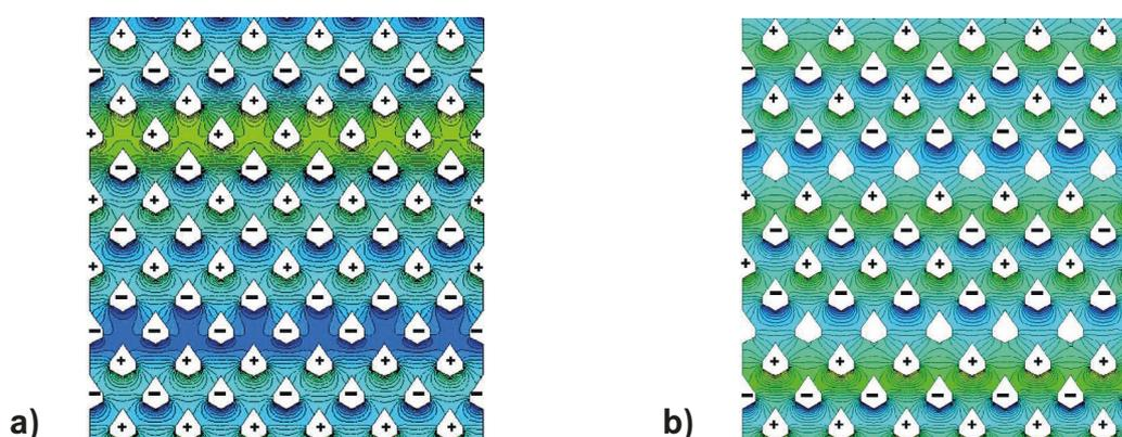
Figure 7: Pressure distribution in the MFD for (a) horizontal configuration of the air ducts with revolved sections and (b) the new design with a row of closed ducts per dryer section simulated with an air flow rate of  $465 \text{ m}^3/\text{h}$
