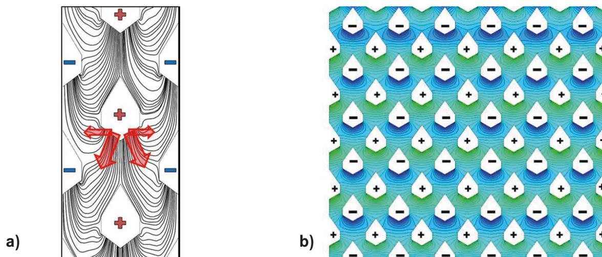
Figure 3: Simulated air flow distribution in the experimental dryer with horizontal configuration of the air ducts: (a) flow line presentation and (b) pressure distribution (static particulate bed; air flow rate of 465 m<sup>3</sup>/h), (+) inlet air and (-) outlet air ducts.
