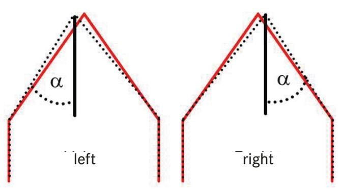
Figure 5: Geometric presentation and qualitative comparison of the original (red line) and the new developed (dotted line) roof geometry
