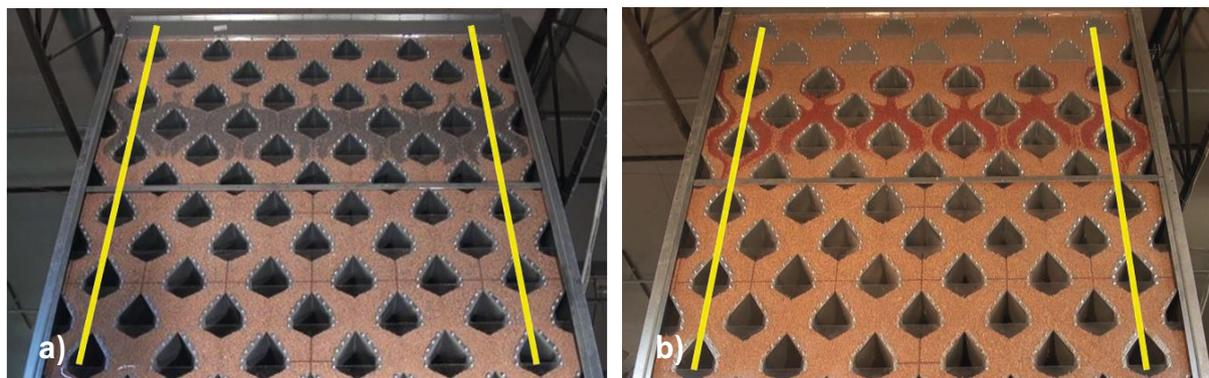
Figure 6: Experimentally measured particle flow profile for (a) conventional air ducts and (b) new developed air ducts (with altered roof angle in the vicinity of sidewalls) (© F. Weigler)
