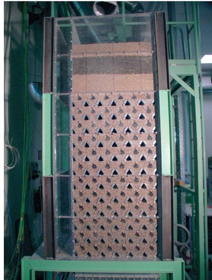
Figure 1: The geometry of the experimental dryer without air inlet and outlet duct hoods for process analysis of particle flow, airflow and the drying process (© F. Weigler)
