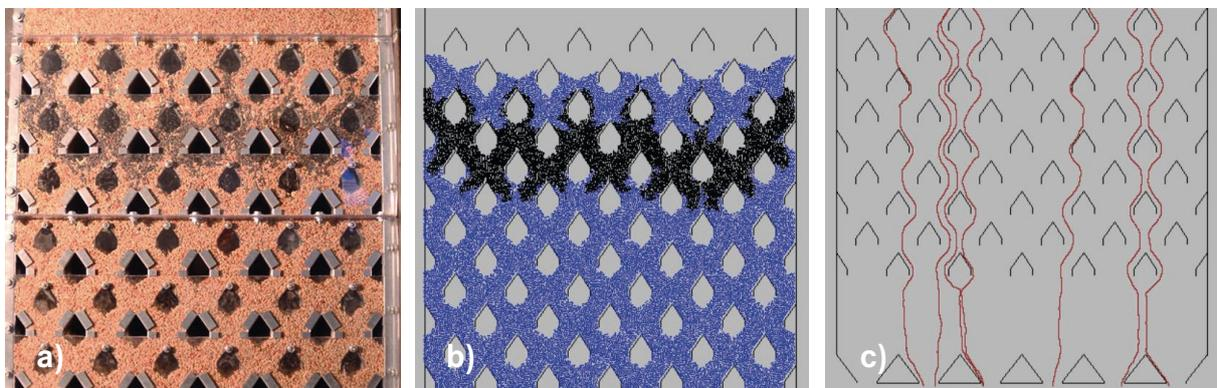
Figure 2: Particle movement in the test dryer: (a) experimental, (b) numerical and (c) particle trajectories
