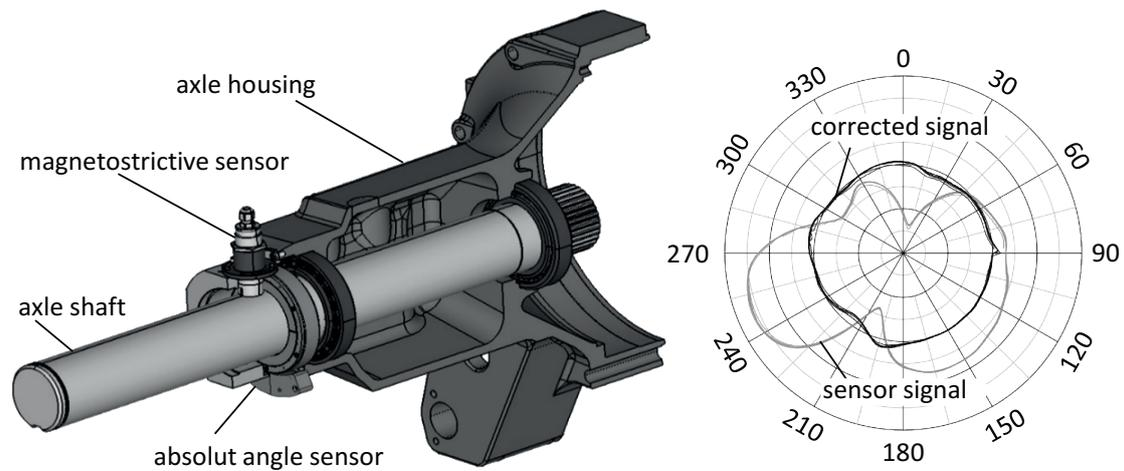
Figure 8: Sensor assembly in the rear axle housing and signal correction via an absolute angle sensor
