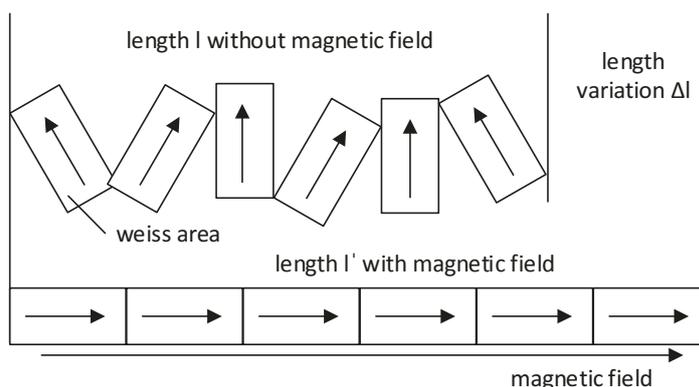
Figure 6: Joule effect: Length variation of a ferromagnetic part caused by a magnetic field (HERING 2012)
