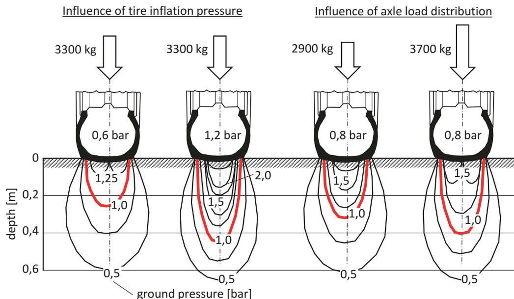
Figure 1: Pressure bulbs beneath a tire Michelin Multibib 650/65R38 on dry secondary podsol (CH7) for various tire loads (left) and various contact area (right), calculated with the soil-compaction-model Terranimo (STETTLER et al. 2014)
