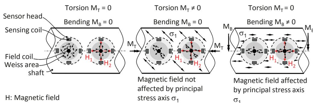
Figure 7: Functionality of a magnetostrictive bending sensor
