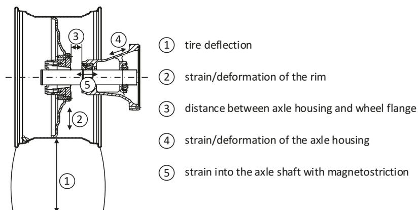
Figure 3: Possible sensor positions and principals for tire load detection on rigid axles
