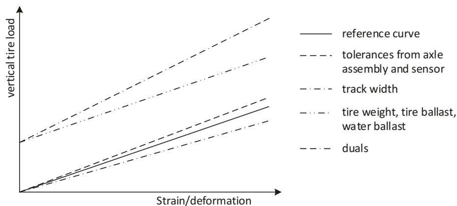
Figure 4: Impact of disturbing factors between force transmission point and tire load sensor on calibration function of the sensor, according AGCO INT. GMBH (2013b)
