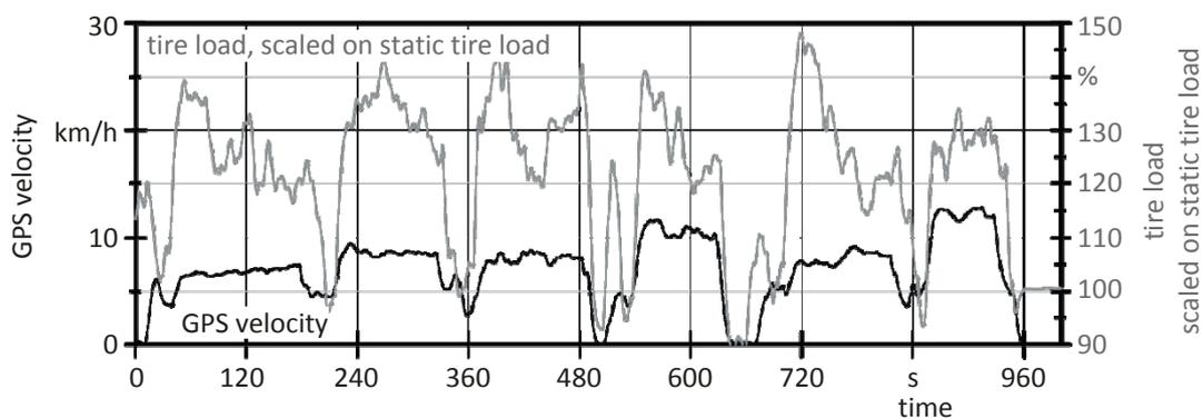
Figure 10: Load on the rear right tire of an Arion 550 equipped with a semi-mounted cultivator and 900 kg front ballast
