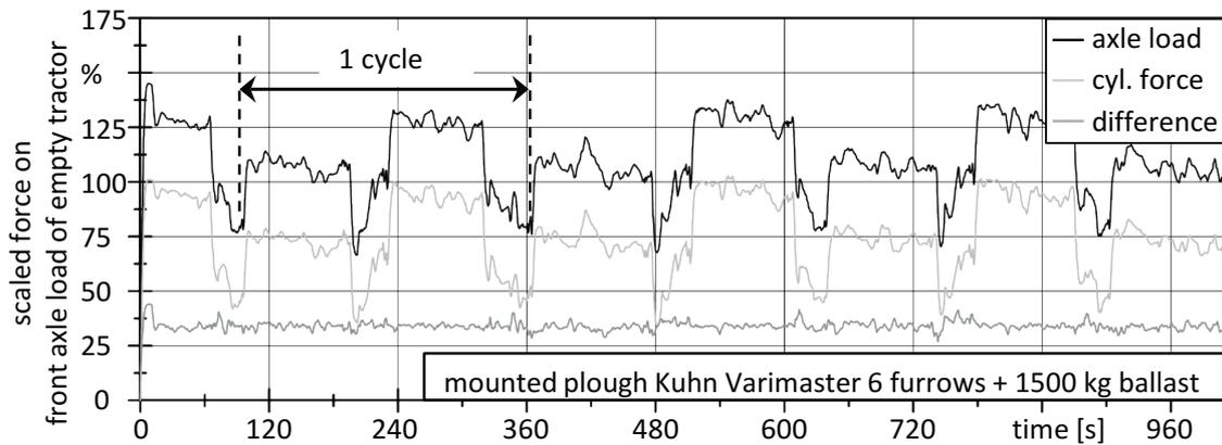
Figure 9: Difference of axle load and calculated cylinder force, measured with an Axion 840 equipped with a 6 furrow plough and 1500 kg front ballast
