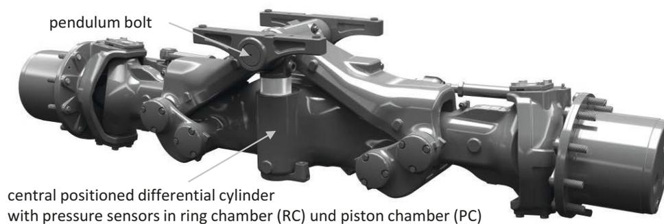
Figure 5: Assembly of a hydropneumatic suspended axle with a central suspension cylinder and pressure measurement
