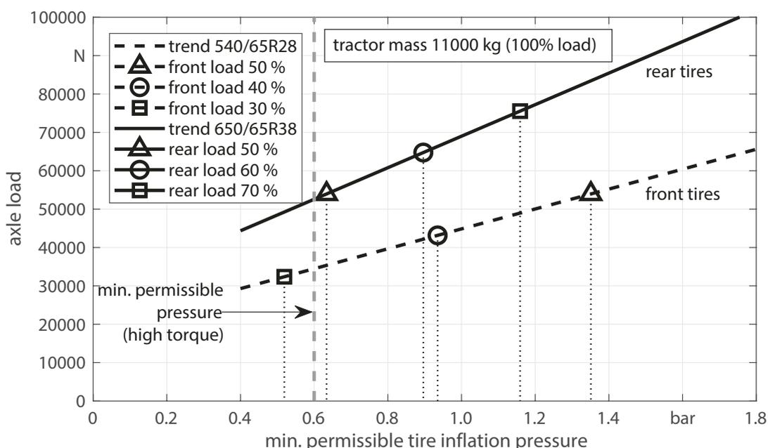
Figure 2: Axle loads (addition of 2 tires) and appropriate minimal tire inflation pressure for various axle load distributions for a middle range standard tractor equipped with Michelin Multibib tires
