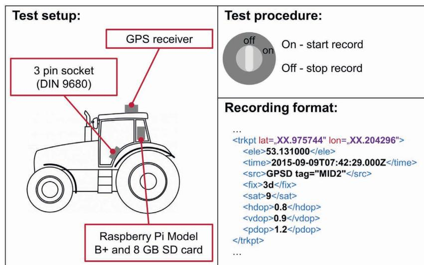
Figure 4: Test setup, test procedure and recording format
