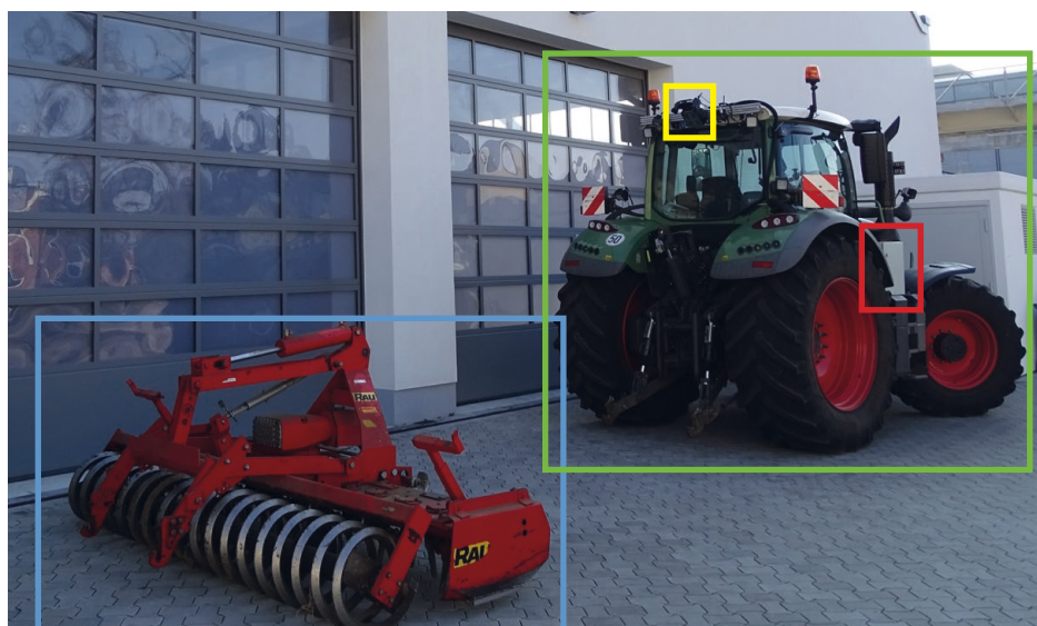
Figure 2: Test setup for coupling to implements (blue: implement, green: test vehicle, yellow: sensor, red: power supply)
