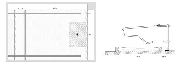
Figure 2: Schematic drawing of the chambers position in the cubicle (left); Lateral view of the cubicle (right, adapted from Sulzberger OHG)
