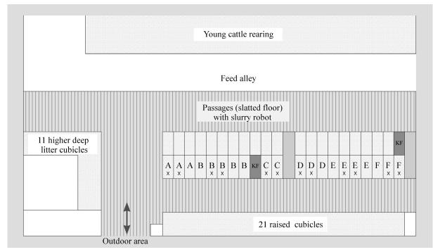
Figure 1: Sketch of experimental barn and the tested cubicles (A-F: cubicles with different organic bedding materials, x: positioning of chamber for gas measurement, KF: concentrate feeder).
