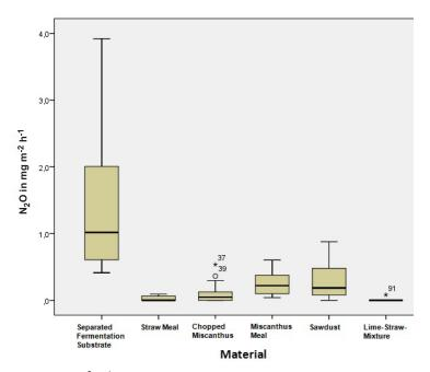
Figure 4: N<sub>2</sub>O emissions in mg m<sup>-2</sup> h<sup>-1</sup> from different scattered cubicles (\*  $\triangleq$  extreme value; °  $\triangleq$  statistical outliers > 1.5 boxlength, bar inside boxplot  $\triangleq$  average)
