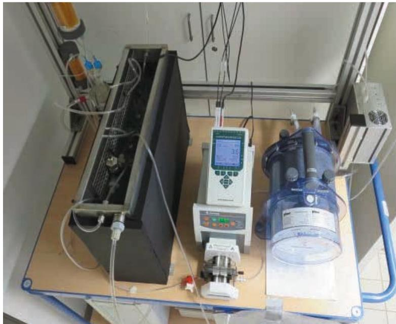
Figure 5: Test equipment for gas cleaning (section) with adsorption columns in the water bath (left), sample gas cooler (rear right) and drying columns (rear left) (© Hochschule Weihenstephan)
