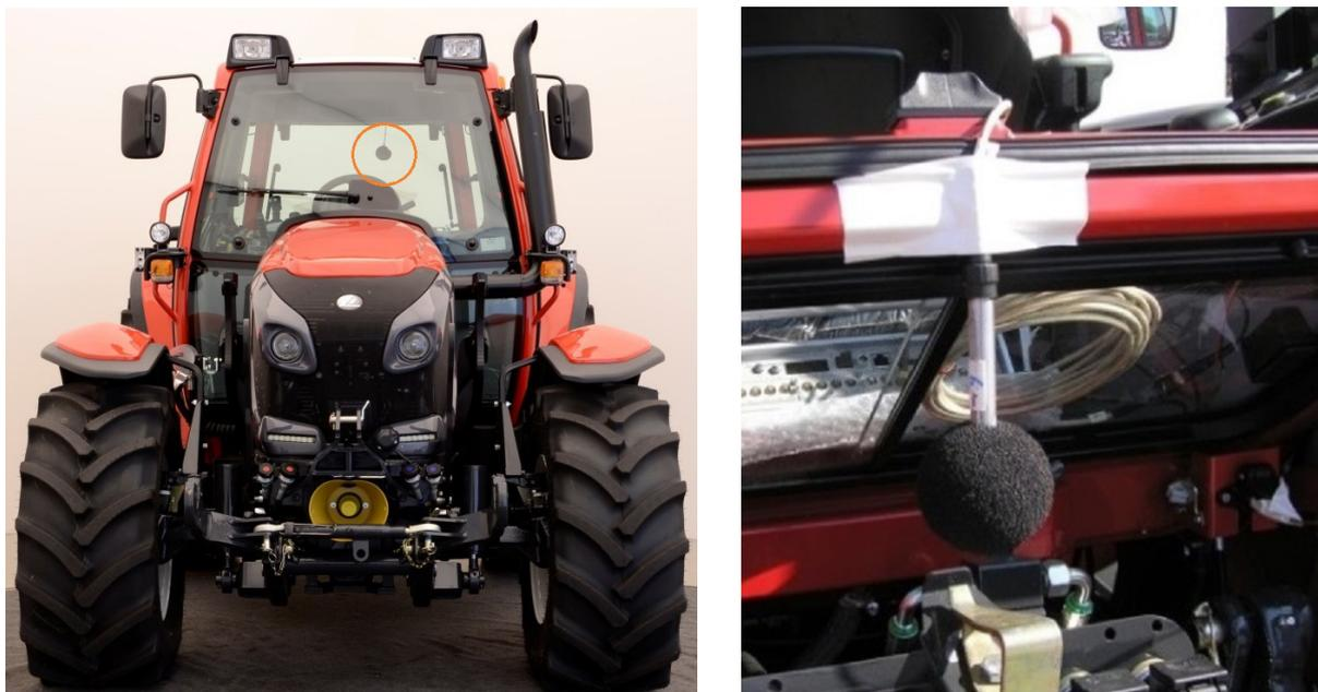
Figure 3: Microphone position (airborne sound microphone driver, airborne sound microphone near field transmission rear) on the Lintrac 90 (Photo: Lindner Traktorenwerk GmbH)
