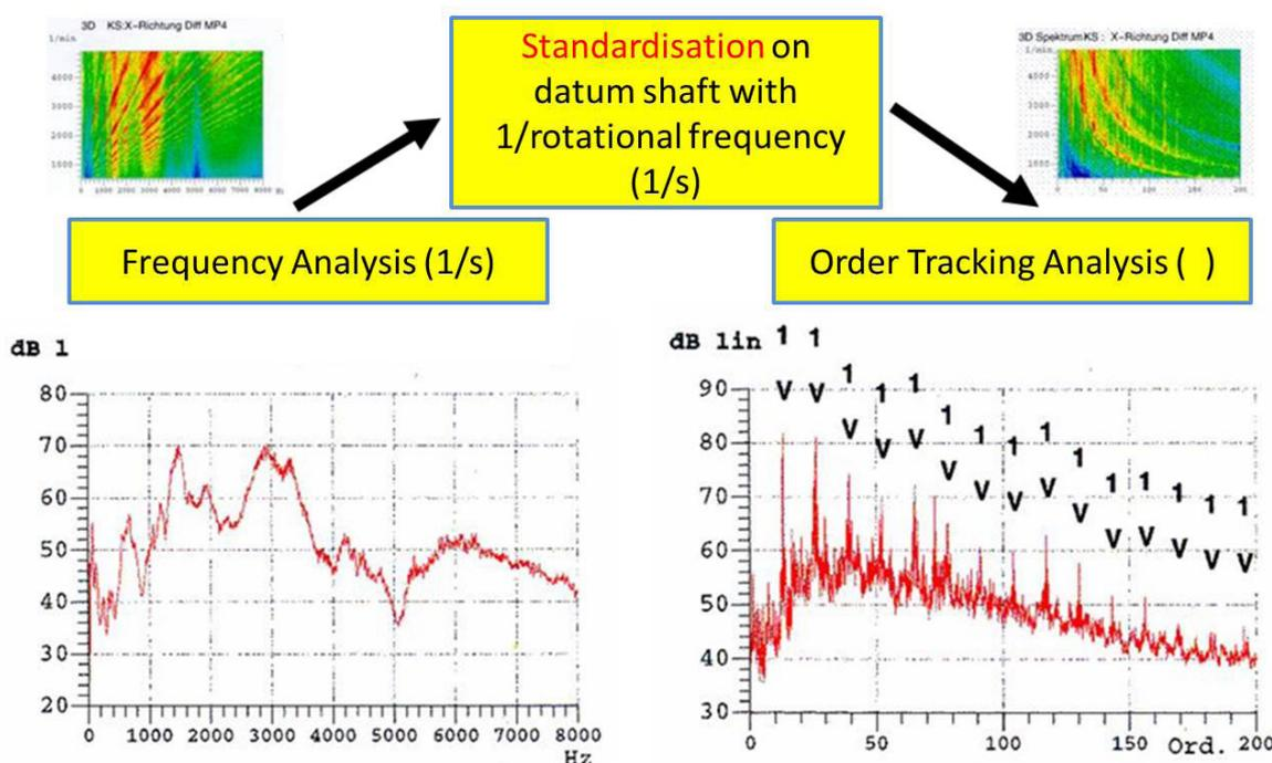
Figure 2: From the frequency to the order tracking analysis (WAGNER 2005)
