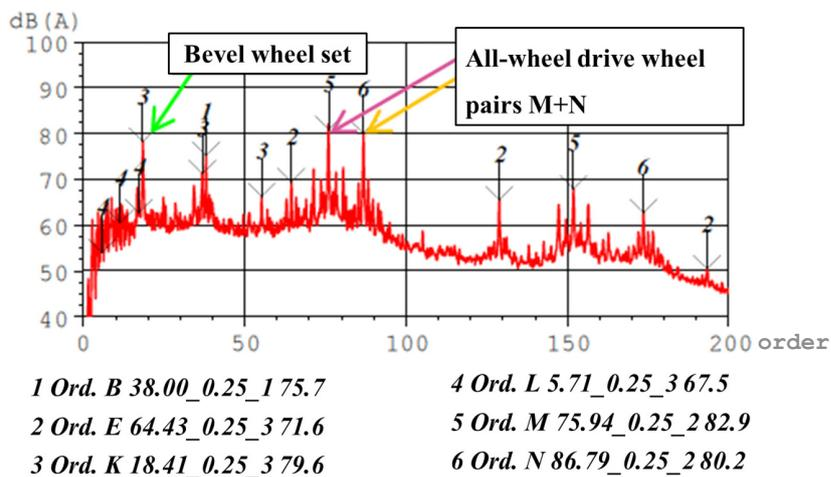
Figure 6: Geotrac recording, order tracking analysis of airborne noise in near field transmission rear
