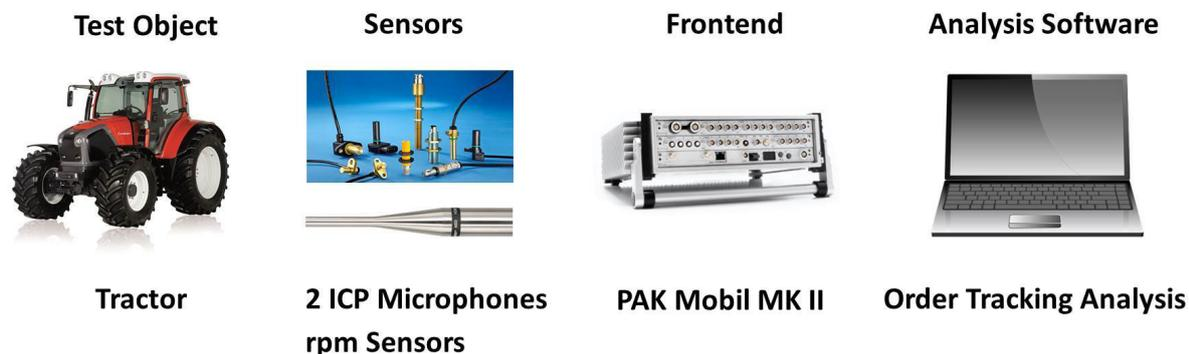
Figure 1: Measurement chain
