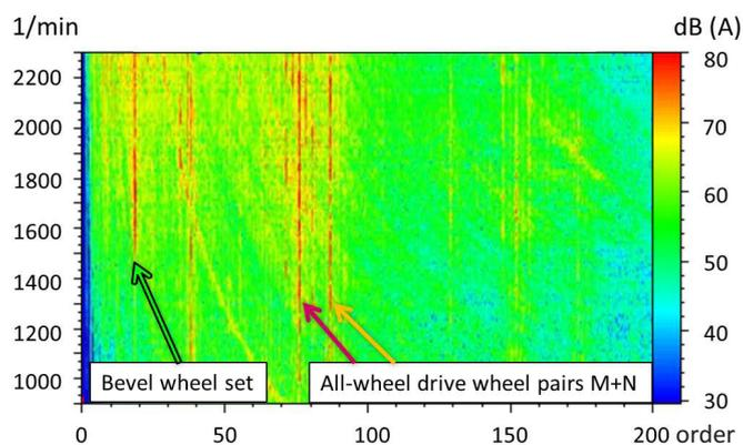
Figure 5: Geotrac recordings, Campbell Diagram of the order analysis (airborne sound in near field transmission rear)
