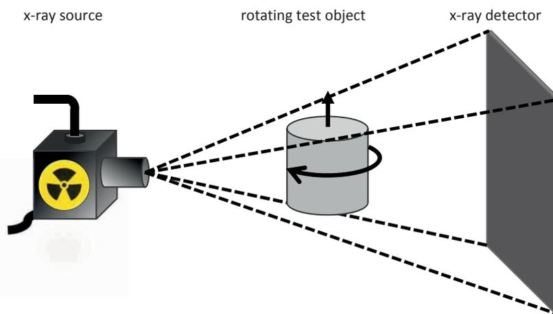
Figure 1: Schematic of an industrial computer tomography
