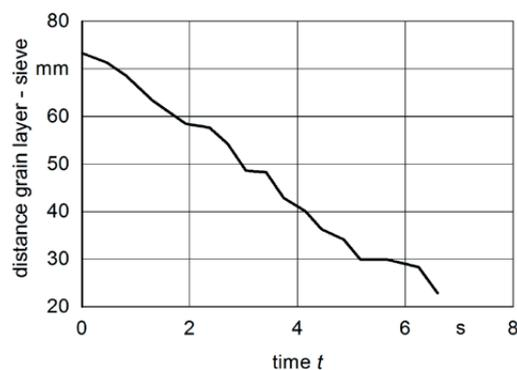
Figure 10: Distance grain layer – sieve in a grain-MOG-mixture during a segregation process determined using the computer tomography
