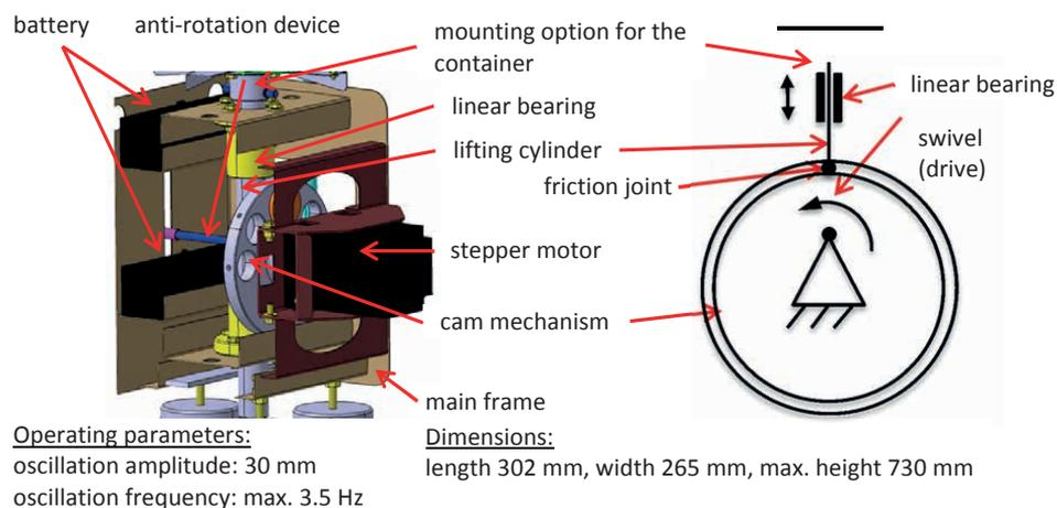
Figure 3: Miniature test rig to generate a vertical oscillation
