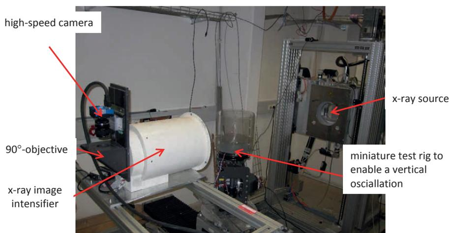
Figure 4: Miniature test rig installed in the CT system
