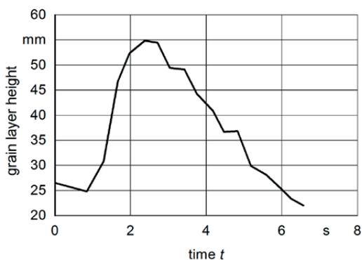
Figure 9: Grain layer height in a grain-MOG-mixture during a segregation process determined using the computer tomography
