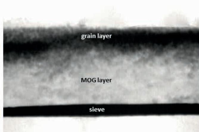
Figure 7: X-ray image of the grain-MOG-mixture at the beginning of the experiment
