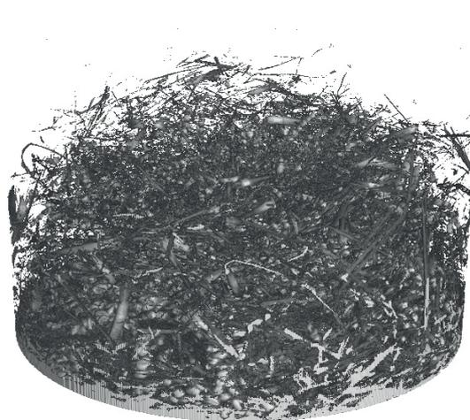
Figure 6: 3D image of the grain-MOG-mixture created with help of the computer tomography; grain and MOG is displayed
