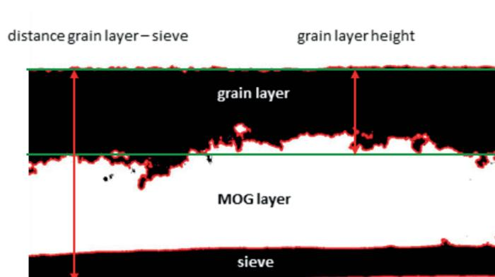
Figure 8: Binary image of the grain-MOG-mixture
