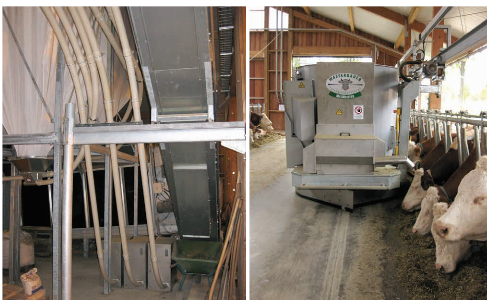
Figure 1: Concentrate feed silos, mineral feed dispensers and conveyor belt, with feed bunkers in the background in the feed kitchen; Feed mixing and distribution wagon with some of the AMS herd (Photos: R. Oberschätzl)
