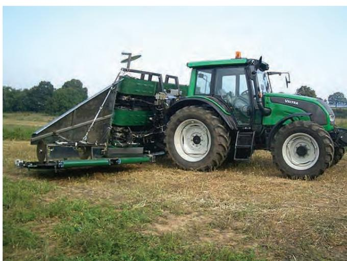
Figure 2: Harvesting machine prototype of the company Kranemann for mowing and cross-parallel laying of hemp stems (Photo: H.-H. Kranemann)
