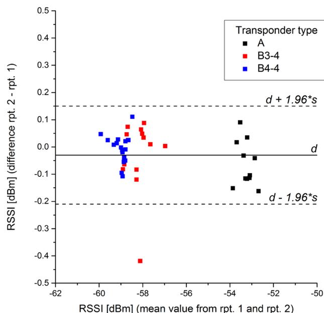
Figure 5: Bland-Altman diagram of trial for determining reproducibility;  $d$  = mean value,  $s$  = standard deviation of the differences between repeats 2 and 1
