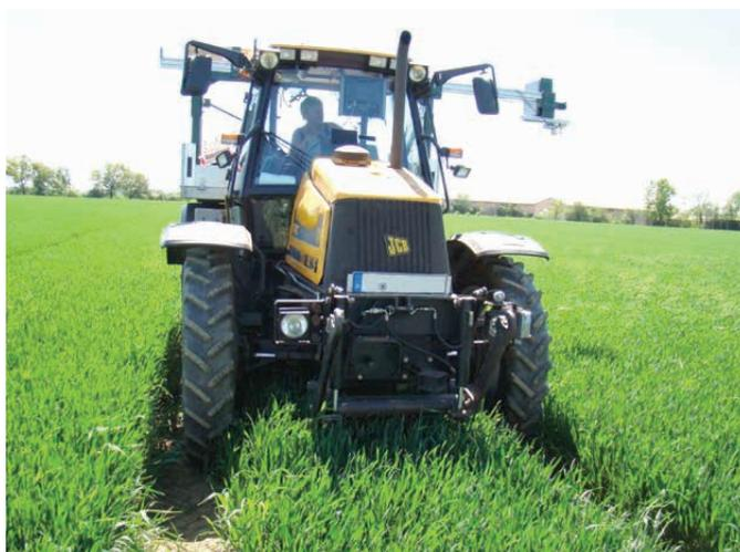
Figure 2: Test prototype of the camera sensor (ATB) in the field trials; operation height: 2.50 m above ground on the left side in the driving direction
