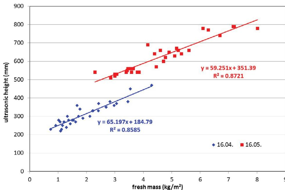
Figure 8: Relationship between the ultrasonic value (“ultrasonic height”) and biomass at the Ostrau II field site at two sampling periods in 2014
