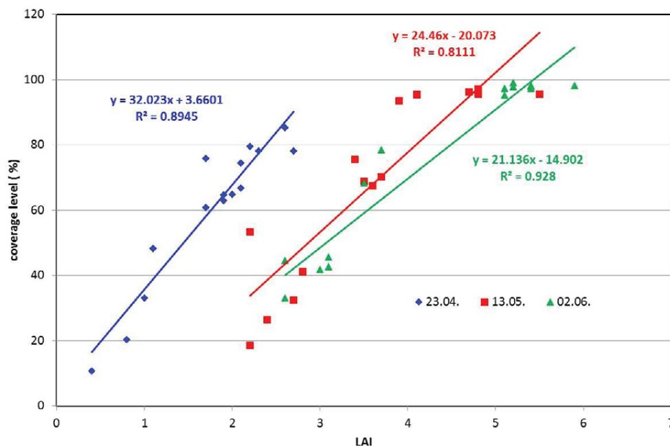
Figure 10: Relationship between the camera value (“green coverage level”) and LAI at the Dabrun II field site at three sampling periods in 2014
