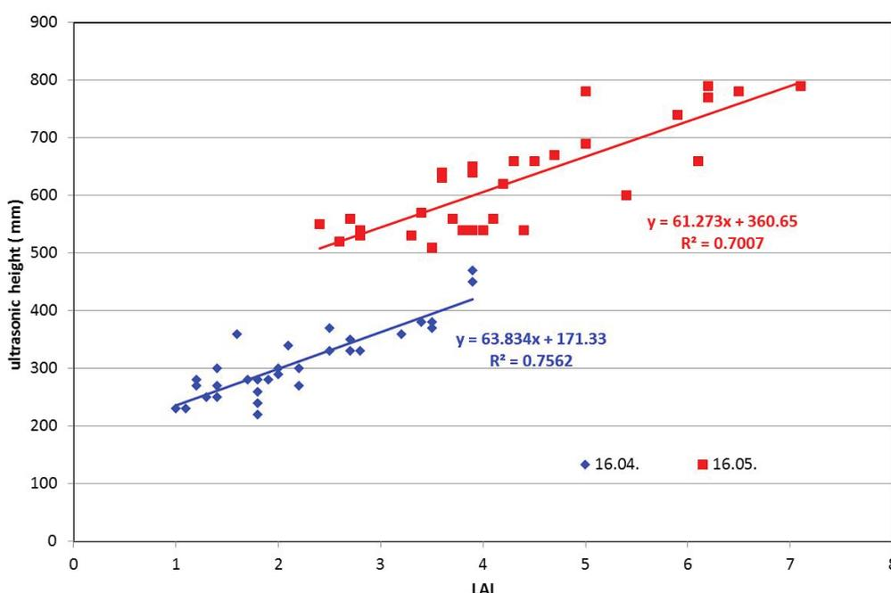
Figure 7: Relationship between the ultrasonic value (“ultrasonic height”) and LAI at the Ostrau II field site at two sampling periods in 2014
