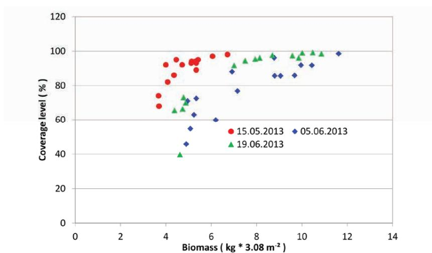
Figure 5: Relationship between the camera value (“coverage level”) and biomass at the Dabrún I field site at three sampling periods in 2013
