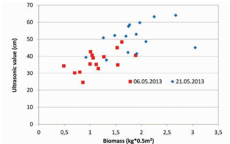
Figure 3: Relationship between the ultrasonic value (“ultrasonic height”) and biomass at the Ostrau I field site at two sampling periods in 2013
