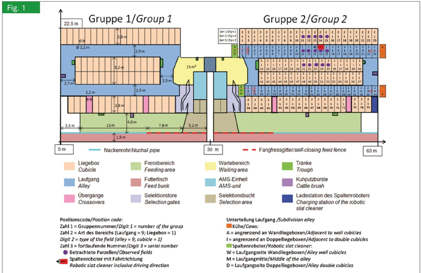
Schematic drawing of the freestall's floor plan including the dimensions, the division into fields and the defined robotic slat cleaner's sphere of influence
