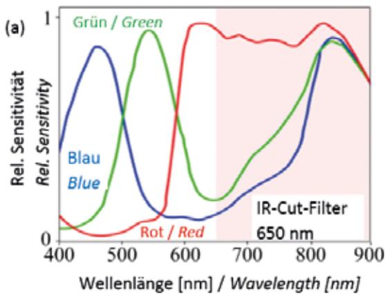
Spectral response of the MT9V032STC CMOS image sensor (IDS datasheet)
