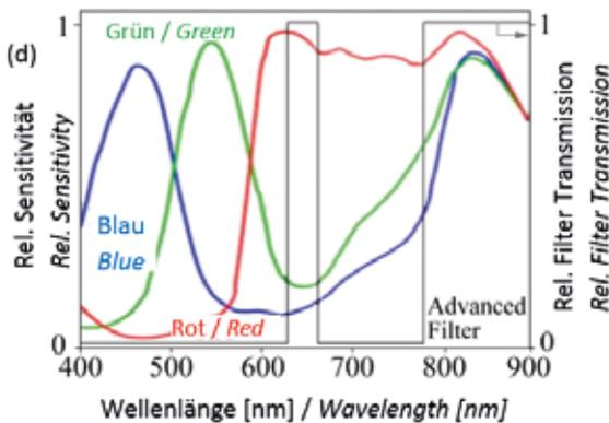
Enabling the RGB CMOS chip for red and NIR sensitivity through ideal double band pass filters
