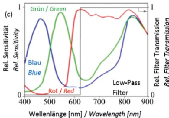
Enabling the RGB CMOS chip for red and NIR sensitivity through ideal low-pass filter
