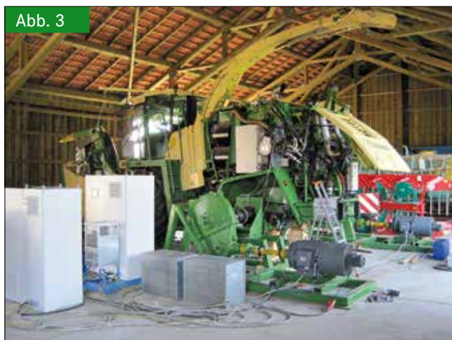
Fig. 3: Test object including test bench components during tests in the experimental hall
