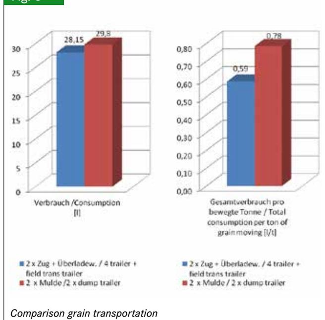
far distance fields. For fields with short distances to the silo the holding times of the crop tractors with two trailers increase sharply. In this case the use of dump trailers is advantageous and generates fuel savings [2].
