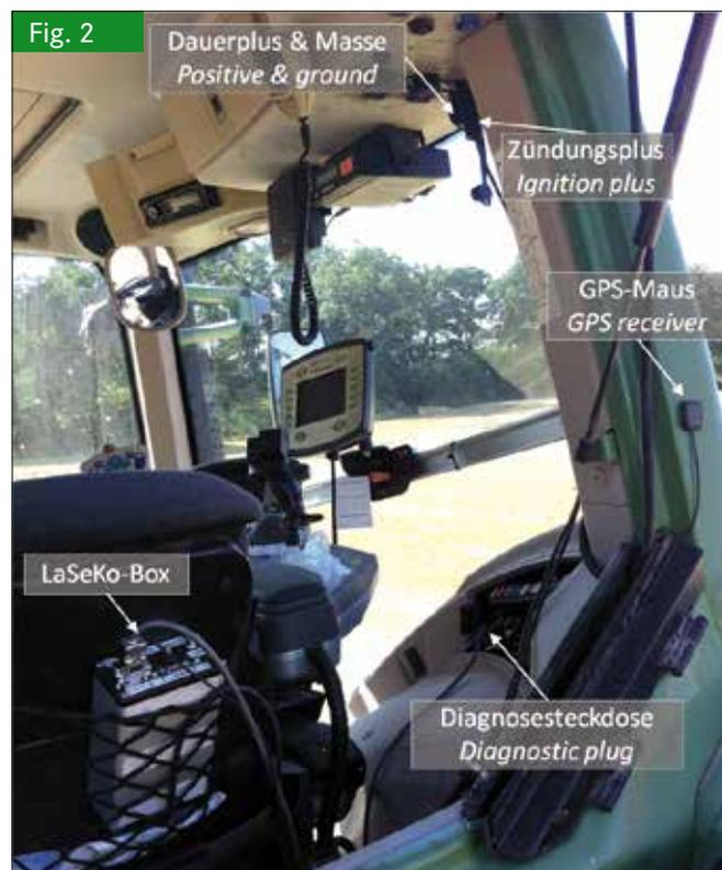
Installed LaSeKo-Box on tractor with plugs (Photo: C. v. Toll)
