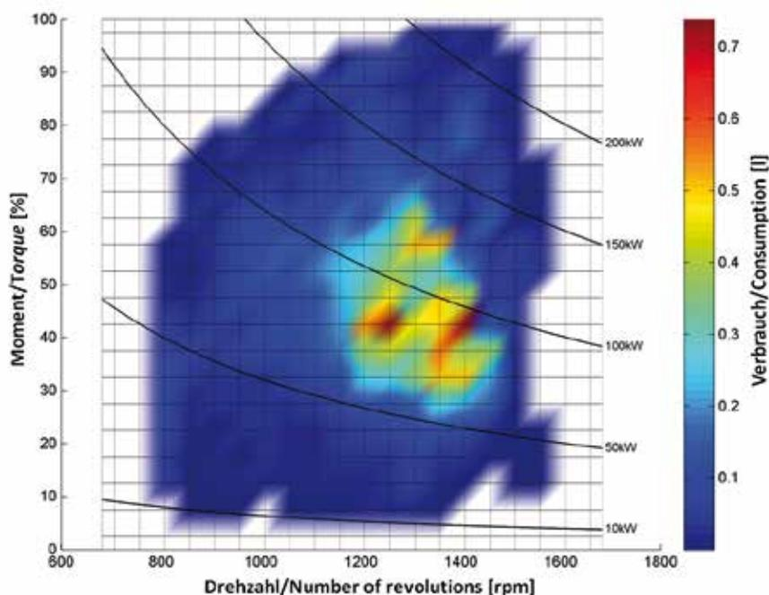
Power chart for fertilizer spreading on 10 ha field, tractor power: 261 kW
