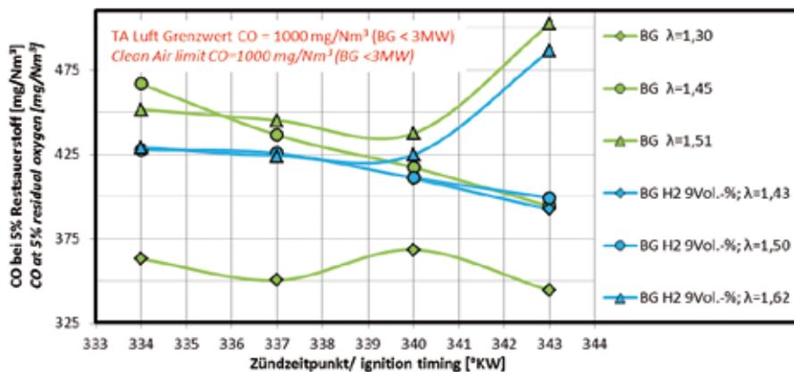
Influence of ignition timing on the CO-Emission of BG 50/50 with 0 and 9 vol.-% H<sub>2</sub> [4]
