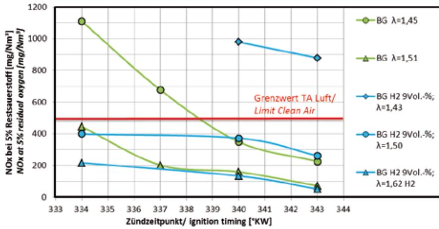
Influence of ignition timing on the NO<sub>x</sub>-Emission of BG 50/50 with 0 and 9 vol.-% H<sub>2</sub> [4]
