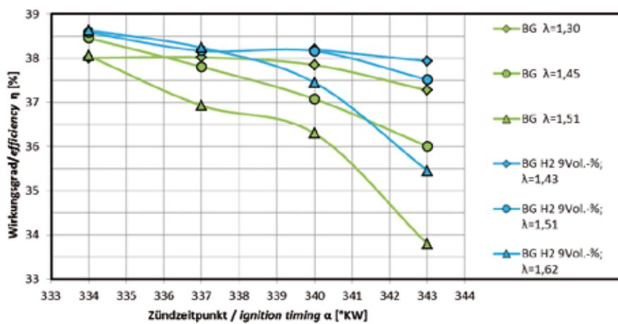
Influence of ignition timing and air ratio on the efficiency of BG 50/50 with 0 and 9 vol.-% H<sub>2</sub> [4]
