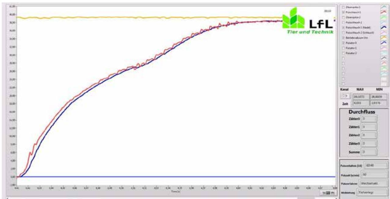
Results of an example measurement (yellow - operating vacuum; red - measuring point within the short pulse tube; blue - measurement with needle and tube (inside diameter  $\varnothing$  4 mm, 30 cm long))
