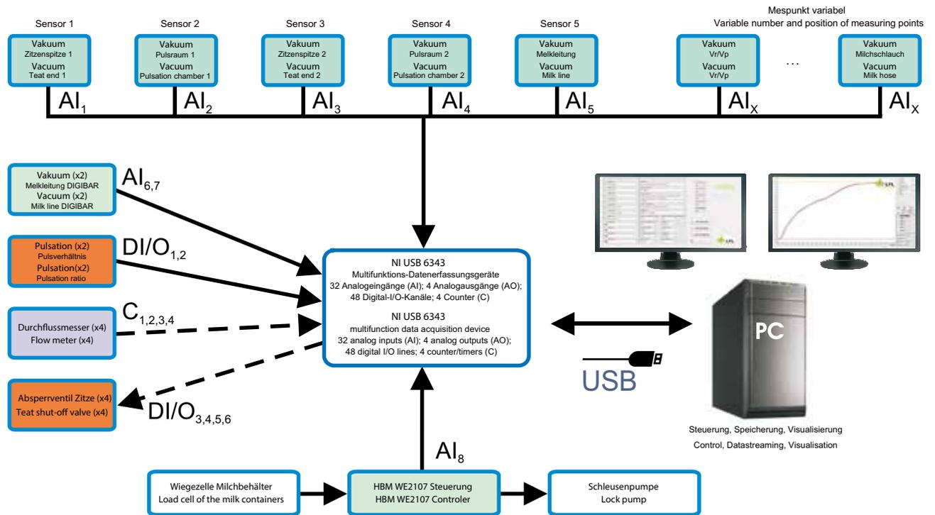
Concept of the milking laboratory with integrated sensors and data acquisition system (— implemented; --- under testing)
