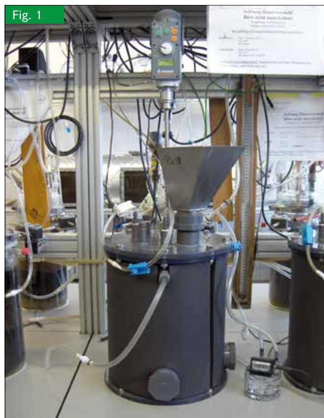
Continuously-stirred-tank reactor with a net volume of 10 l (photo: C. Beil)
