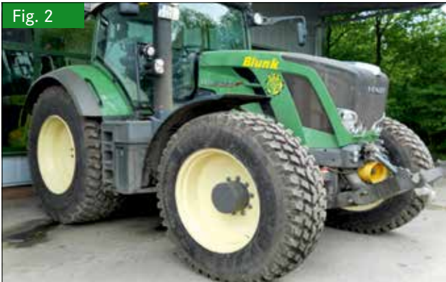
Fendt Vario 828 with industrial tires (Nokian TRI2)
