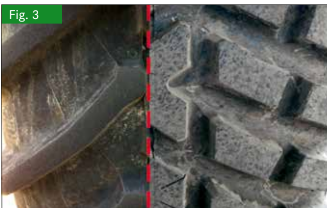
Comparison of AG tires (left) and industrial tires (right) (Foto: Reckleben)
