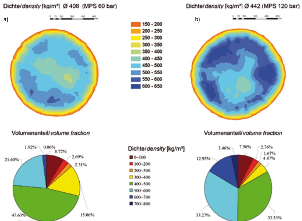
Density distribution of the bale profile and volume fractions of the different density classes in case of pressing with a) maximal and b) minimal pressure adjustment of the MPS, Silage crop 35-45% DM
