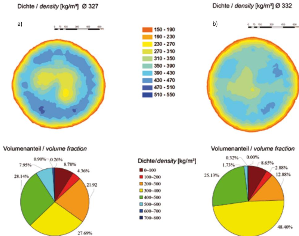
Density distribution of the bale profile and volume fractions of the different density classes in case of two different baler types a) Rollant 374 and b) Rollant 455, Silage crop 45-55 % DM
