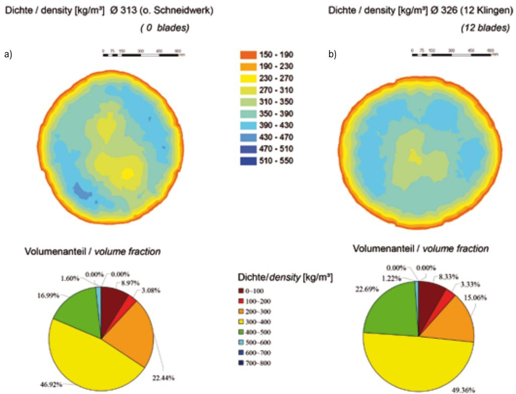
Density distribution of the bale profile and volume fractions of the different density classes in case of pressing a) with 12 blades and b) without blades, Silage crop 50-55 % DM
