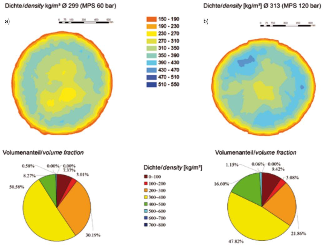
Density distribution of the bale profile and volume fractions of the different density classes in case of pressing with a) maximal and b) minimal pressure adjustment of the MPS, Silage crop 50-55% DM
