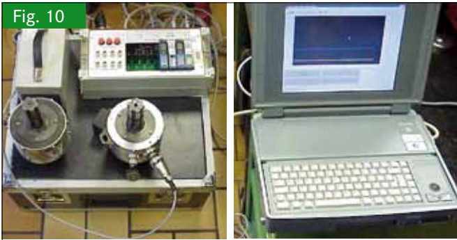
Measuring hubs, amplifier and recording equipment (left), computer-aided evaluation unit (right) (Photo: GKN Walterscheid)
