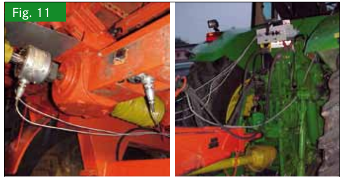
Field measurement; arrangement of the measuring hub for torque and speed and wiring to the tractor (Photo: GKN Walterscheid)
