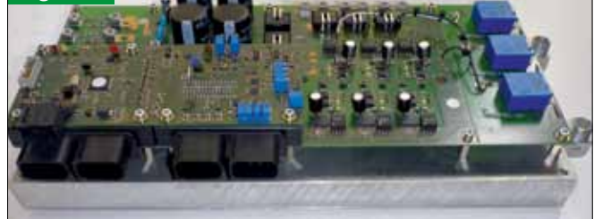
30 kVA high power inverter for agricultural applications (Photo: TU Wien)
