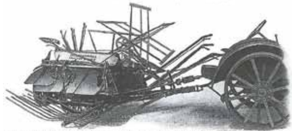
Illustration 206. 10-ft. Tractor Binder and International Tractor. The handle, cutter, power take-off of the tractor are not included with the binder in weight or price.
