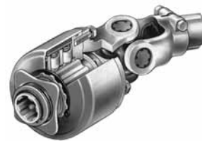
Cam-type friction clutch 1600 Nm, year of construction 1958
