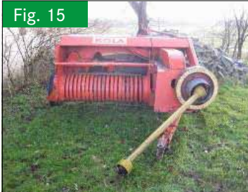
Coil-spring friction clutch 550 Nm, year of construction 1958
