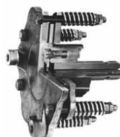
Combined friction and overrunning clutch 1500 Nm, year of construction 1964
