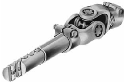
Cam-type ratchet 400 Nm, year of construction 1953/54
