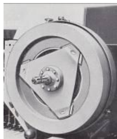
Welger flywheel clutch, year of construction 1968
