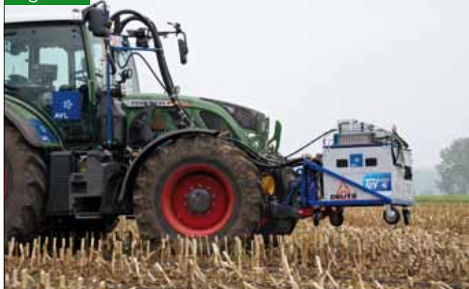
Application of PEMS on the vehicle (Fendt 720 Vario) (Photo: Mathies)
