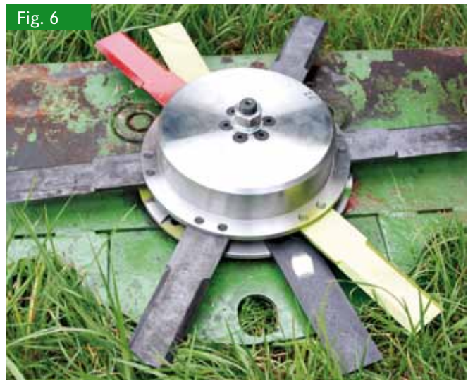
Cutting unit mounted on the mower bar
