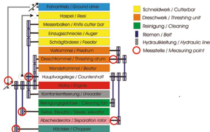
Schematic measuring point plan of the test combine harvester Lexikon 470
