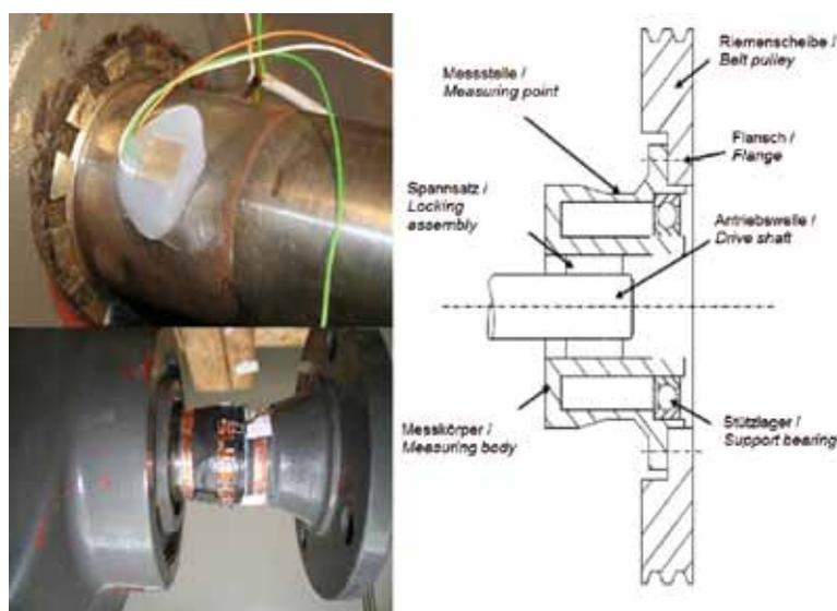
Top left: shaft of threshing drum with strain gages under silicon; bottom left: shaft of rotor gearbox with a rotor electronics; right: sketch of measuring hub of the chopper [2]
