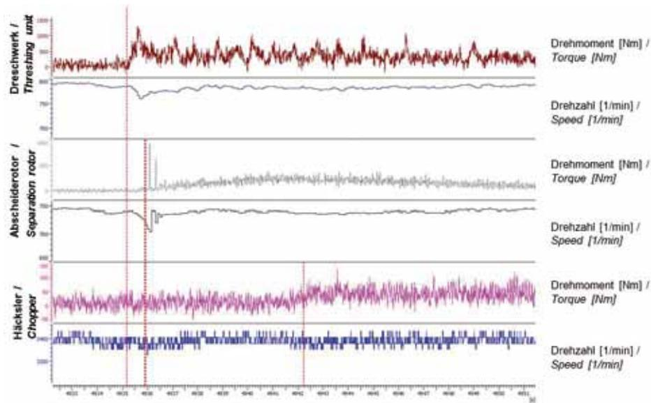
Torque and speed of the threshing unit, the rotor and the chopper during field tests with winter wheat
