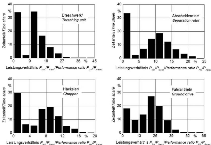
Time share of the measured performance of threshing unit  $P_{DW}$ , rotor  $P_{RO}$ , chopper  $P_{HA}$  and ground drive  $P_{FA}$  related to rated engine performance  $P_{Rated}$
