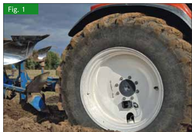
Wheel load measurement in the plough furrow
