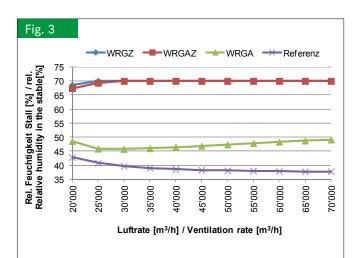
The relative humidity of the reference stable and of the WRGA is considerably lower than in the case of the other two options. 50 %thermal efficiency of the heat exchanger
