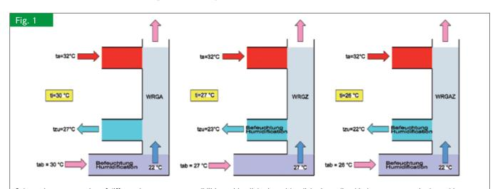
Schematic representation of different heat recovery possibilities, with adiabatic and/or diabatic cooling (ti: the temperature in the stable, ta: the outside temperature, tzu: the temperature of the incoming air, ta: the temperature of the exhaust air)
