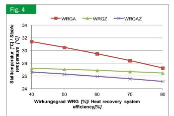
The influence of the thermal efficiency of the heat exchanger on the stable temperature in the case of the three heat recovery systems. Ventilation rate  $40\,000~\text{m}^3/\text{h}$
