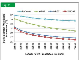
Stable temperature for the 3 types of heat recovery systems in comparison with the reference stable 50 % thermal efficiency of the heat exchanger
