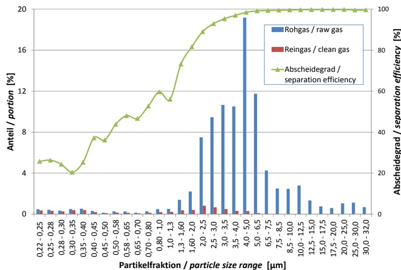
Particle separation efficiency by test facility 1, means from 45 single measurements
