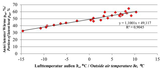
Portion of latent heat at the heat consumption ( $p_{lat}$ ) by air exchange as a function of outside air temperature (mean values from 22 pm to 5 am, 26.01. - 13.03.2012)
