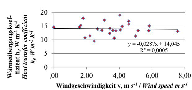
Heat transfer coefficient inside the roof ( $h_i$ ) (mean values from 22 pm to 5 am)
