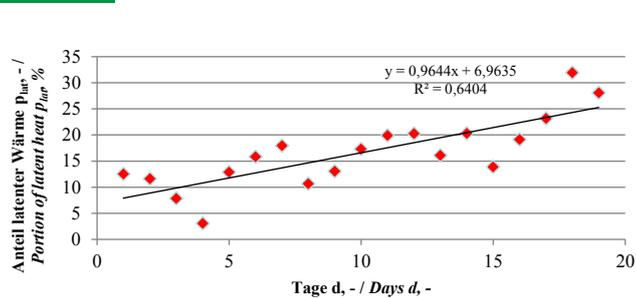
Portion of latent heat at the heat transfer (plat) inside the roof (mean values from 22 pm to 5 am) (days 1 to 4 without a crop, from day 5 with new potted plants)
