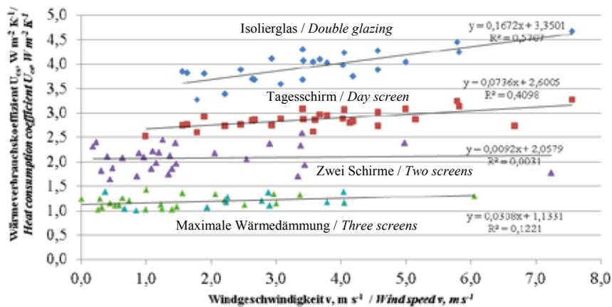
Heat consumption coefficients  $U_{cs}$  as a function of wind speed (mean values from 22 pm to 5 am)
