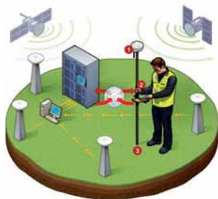
RTK network - schematic, 1 connect, 2 correct, 3 measure
