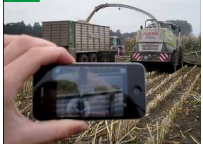
The real time picture of the WLAN camera provided to the whole forage harvester convoy
