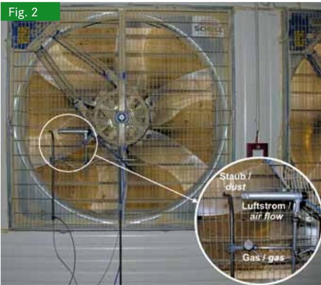
Localisation of the PM sampler in front of an exhaust opening
