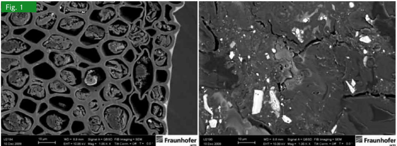
Cut (finley chopped) substrate (left) and extruded substrate (right)
