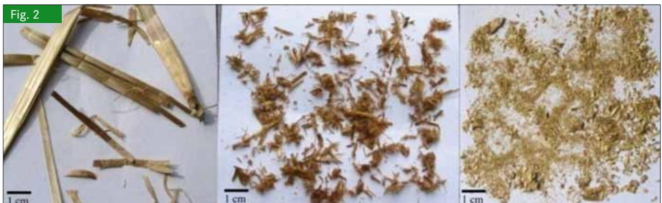
Untreated (left), wet extruded (middle), and dry extruded straw (right)
