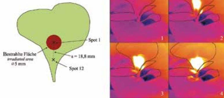
Irradiation tests and thermal images of leaves (*A. retroflexus*); left: 1 laser and 12 measure spots; right: during stationary laser irradiation with 11 W (1: before start, 2: after 5 s, 3: after 10 s, 4: after 15 s) (Drawing, photos: Ch. Marx)
