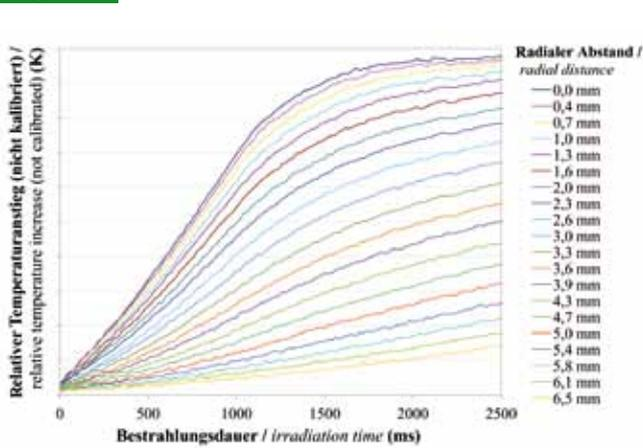
Presentation of thermal measurements with radial distance to the aim spot center during constant irradiation (CO<sub>2</sub>-laser, λ = 10 600 nm, 3.5 W)
