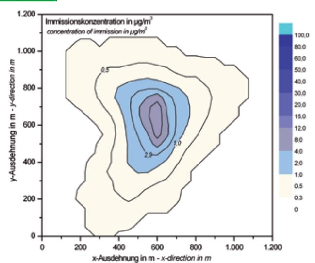
Display of contour lines of ammonia concentration at  $\beta = 355^\circ$
