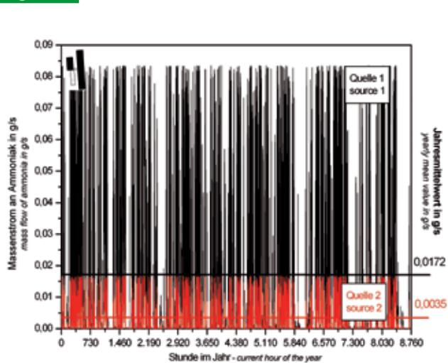
Emission massflow as function of time. Specified are the hourly values during one year of the two box stables of figure 1 at  $\beta = 265^\circ$
