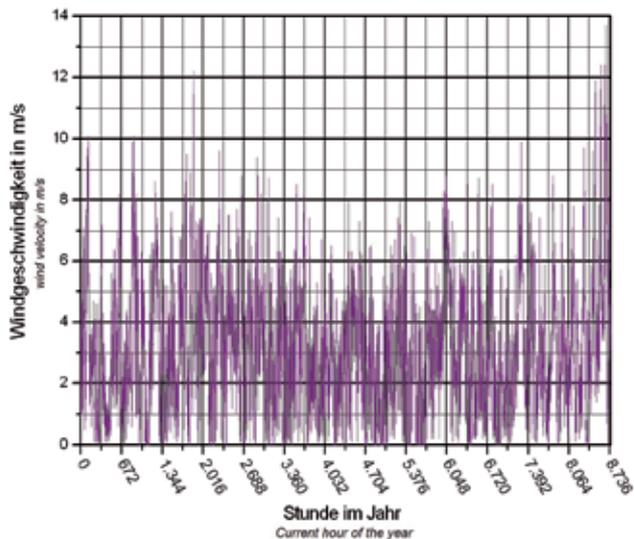
Wind velocity as a function of the current hour of that year that is representative for the selected site. Such data files are produced by Deutscher Wetterdienst (German Weather Service)
