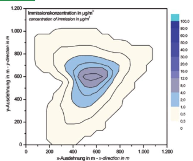
Display of contour lines of ammonia concentration at  $\beta = 265^\circ$
