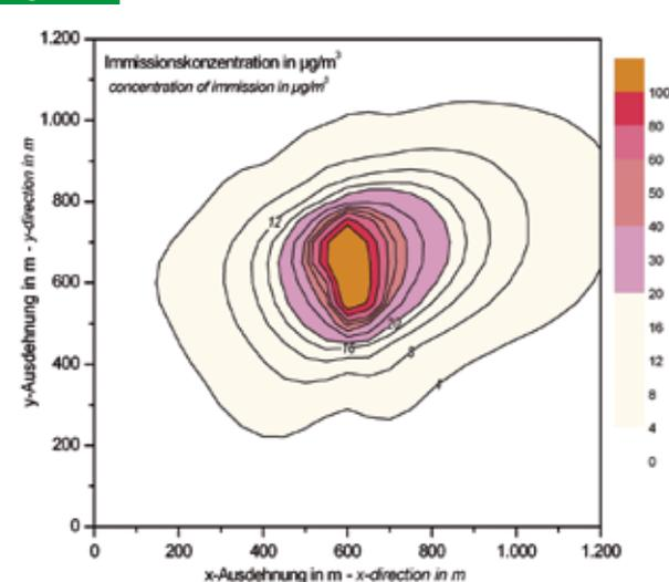
Isolines presentation of ammonia concentration. According to the wind frequency the expansion expand further to north-east than to south-west
