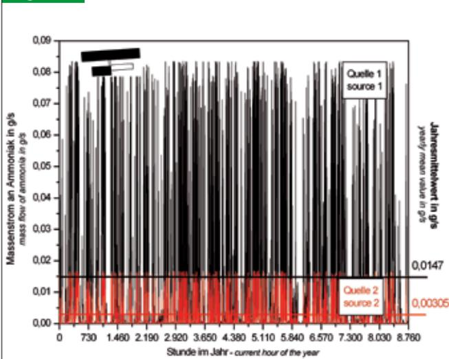
Emission mass flow as function of time. Specified are the hourly values during one year of the two box stables of figure 1 at  $\beta = 355^\circ$
