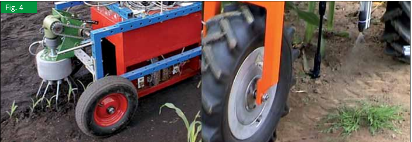
Mechanical weed control within the row (intra row, „Querhacke“, [13]) (left) and weed robot survey „Weedy“ for selective chemical weed control in a field test (right, [14])
