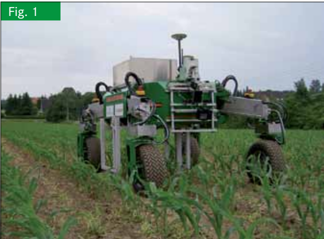
Measurements of individual plants on a maize field with the autonomous field robot BoniRob
