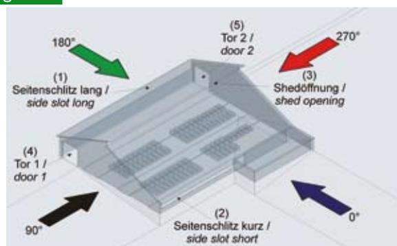
Planned box stable with openings at the end of the feed alley (4), (5), in the sidewalls (1), (2) and in the roof (3). The arrows show the direction of the incoming wind
