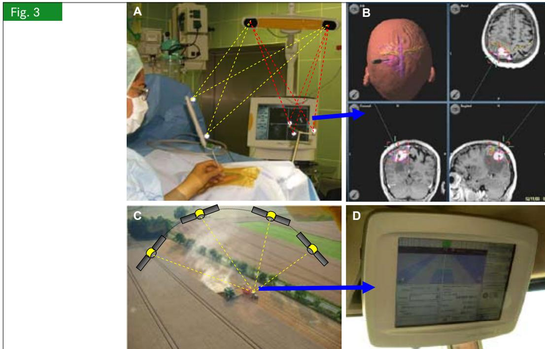
Fig. 3 A: Referencing of a modern frame-less stereotactic system in the operating room. Instruments and reference markers are tracked by a 3-D infrared camera. The yellow lines show the visual axis between camera and instrument, while the red lines show the visual axis to the reference point of the system
